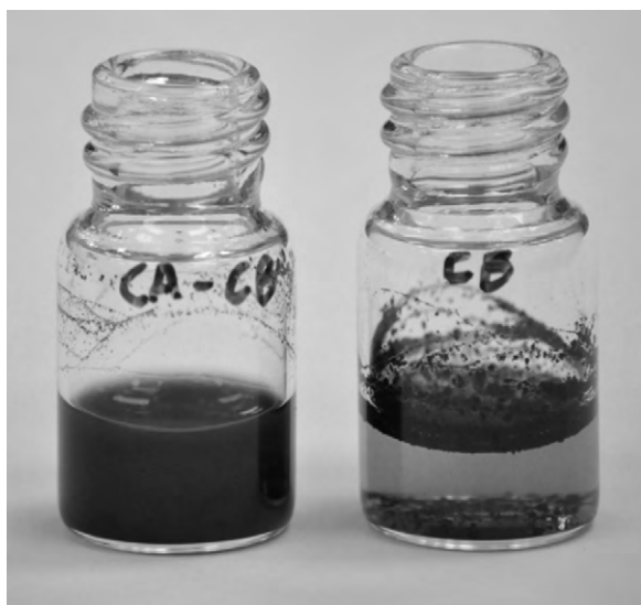
Fig. 4. Comparison of dispersion of 10 mg of citric acid treated XC-72R (CA-CB) and as-purchased Vulcan XC-72R (CB) in de-ionized water after ultrasound treatment for 30 s.
